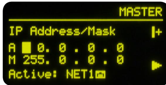
Figure 18 - IP Address Configuration
